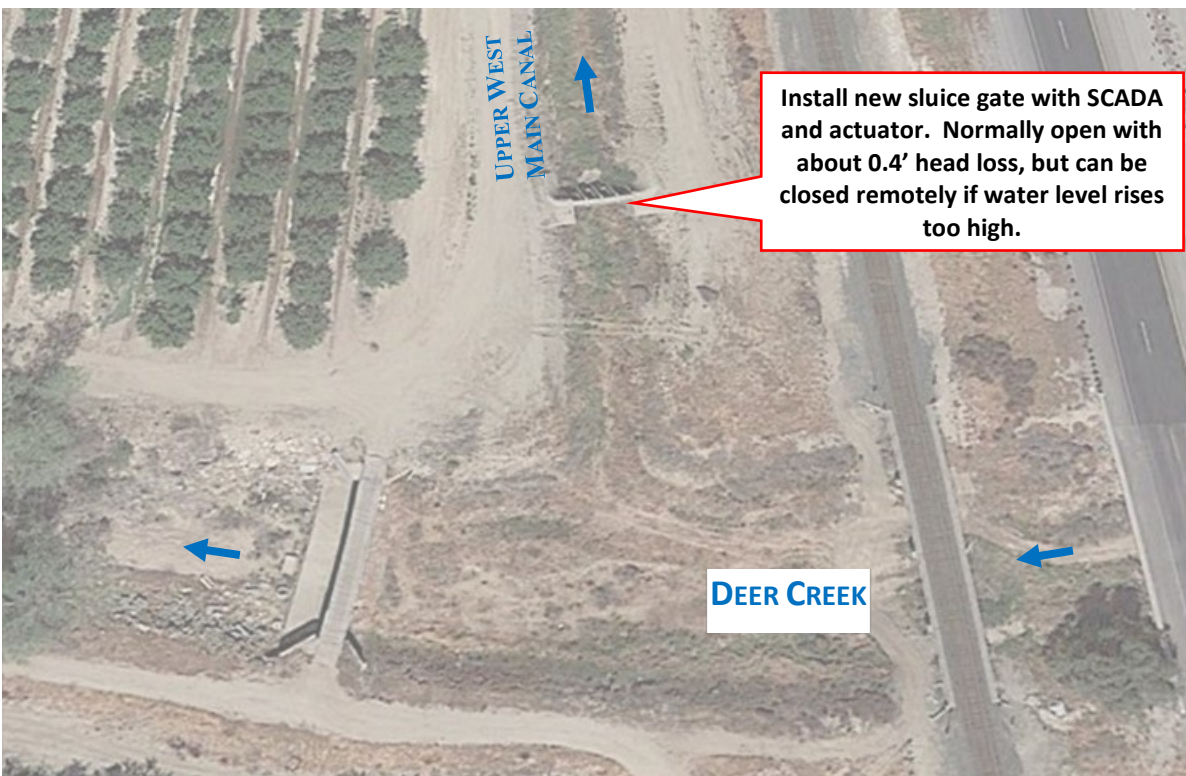
Figure 33. Proposed modifications at Upper West Main Canal and Deer Creek
