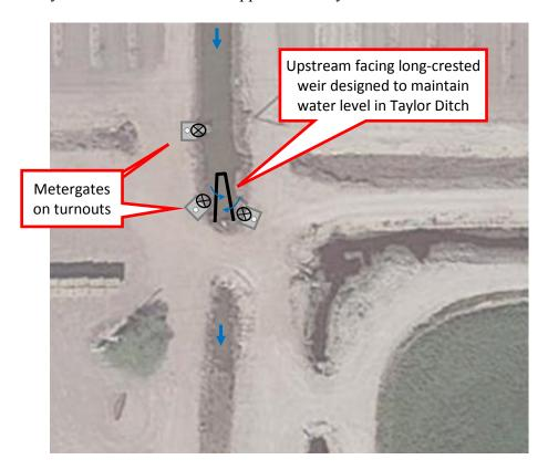
Figure B-37. Layout of option 1 for the Site 5 on the Taylor Ditch
