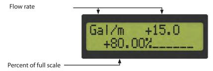
Figure 14: Display Cycle Four
