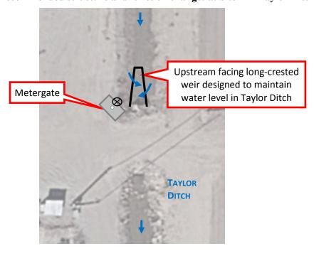
Figure B-25. Recommended structure layout at Site 4 in Taylor Ditch
