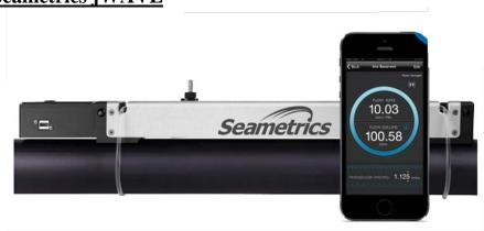
The Seametrics jWAVE Portable Clamp-On Ultrasonic Flow Meter is a portable, non-intrusive flow measurement device. The device clamps on a pipe and connects to a smartphone or tablet via Bluetooth for programming and flow measurement. The manufacturer's literature appears to state that the smartphone or tablet can recall previous settings based on location (i.e. each time you come back to a site, your phone or tablet will automatically recall the pipe type, wall thickness, etc).
