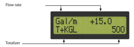
Figure 13: Display Cycle Three
