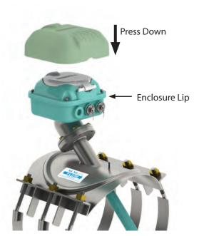
Figure 7: Boot Installation
