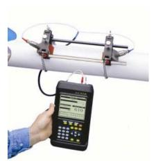
The Panametrics TransPort PT 878 Portable Clamp-On Ultrasonic Flow Meter is a portable, non-intrusive flow measurement device. The device clamps on a pipe and is connected to a wired, handheld unit for programming and flow measurement.
