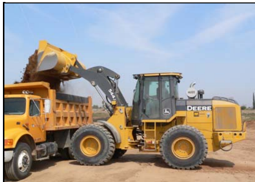
Loader fills District trucks for canal bank repair while dozer works a dam in the river channel.
