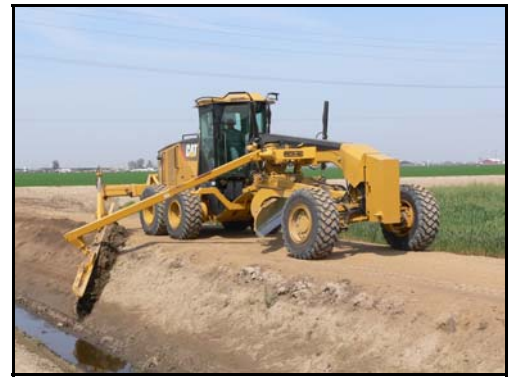
Excavator dips a local sump while an M-Series grader slopes a canal using new ROME blade.
